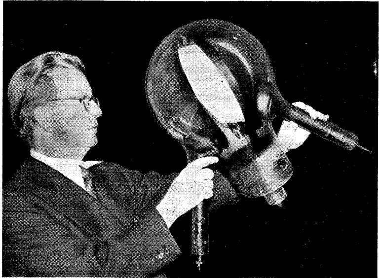
With this type of cathode-ray tube, in which the picture may be viewed on both sides of the screen, the potential size of the audience is doubled.
